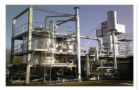
The system shown here features a fixed bed gasification vessel with drying, pyrolysis and gasification stages followed by a WESP to clean and condition the syngas, and an engine/ generator producing CHP. energy transmission and waste disposal.
